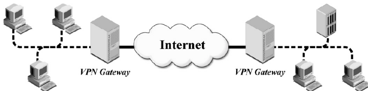
Figure 2-2. Gateway-to-Gateway Architecture Example
