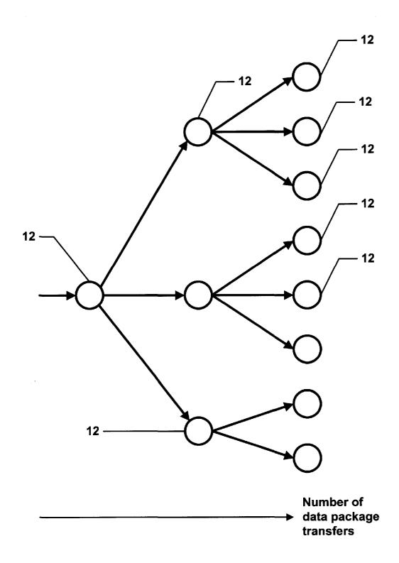
FIGURE 3: Tree-shaped data-flow (optimal)
