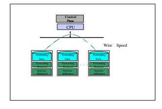
Figure 2: Achitecture of the Accelar Router
