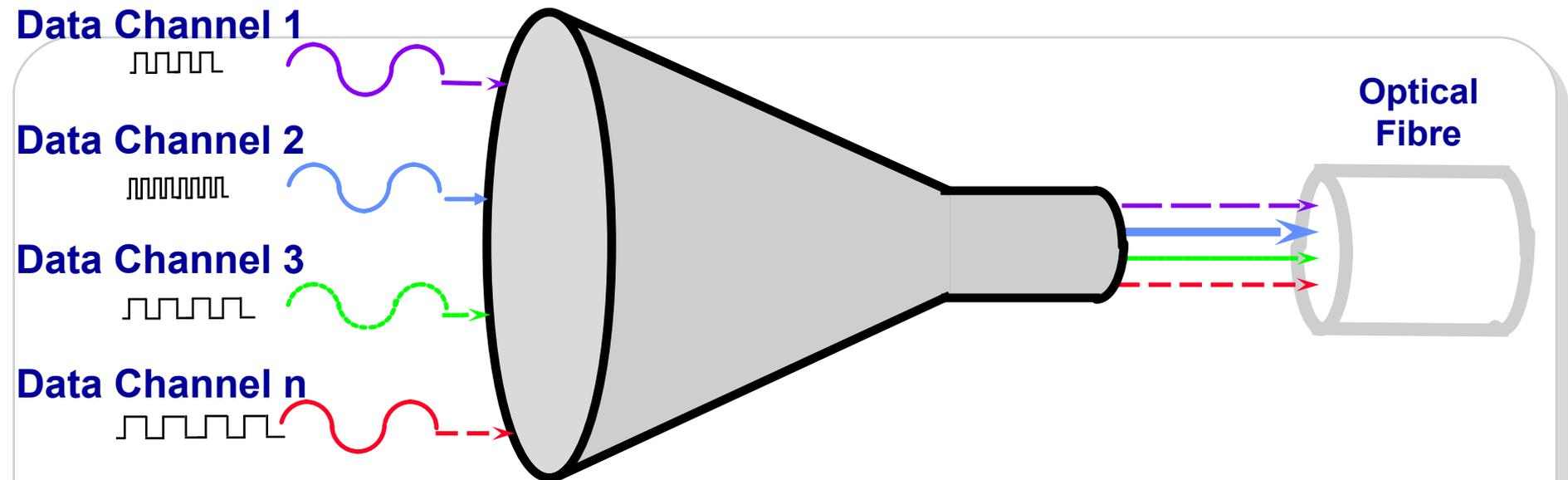
Wavelength Division Multiplexing (**WDM**) acts as “optical funnel” using different colors of light (wavelengths) for each signal
