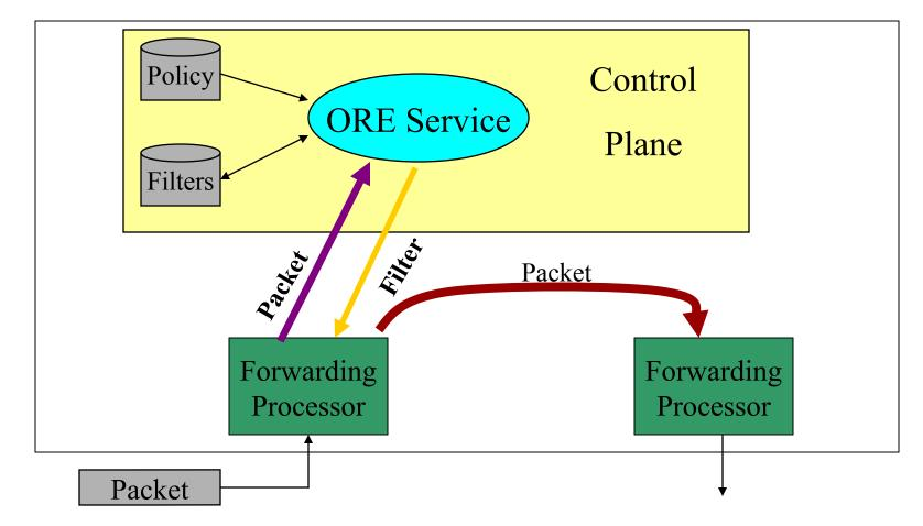
Sample packets, set filters to modify DS-byte for Per-Hop-Behavior modification
